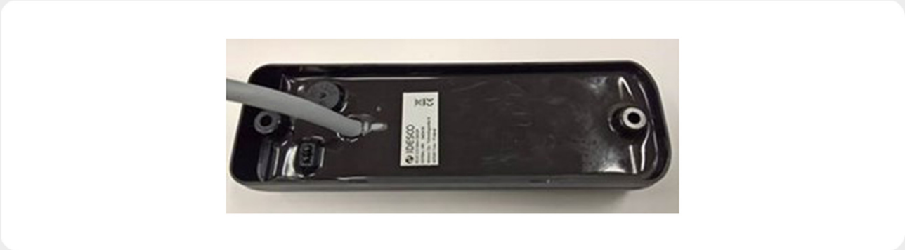
Epoxy filling inside the reader
