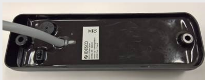
Epoxy filling inside the reader
