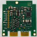
Compact Module 40,9 x 39,0 mm
