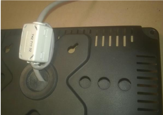
Picture 4 Second ferrite installation
